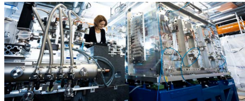
Under pressure: the HED experimental station will be used to study matter under extreme conditions, including new extreme-pressure phases, solid-density plasmas and phase transitions of complex solids in high magnetic fields. (Courtesy: European XFEL/Jan Hosan)
