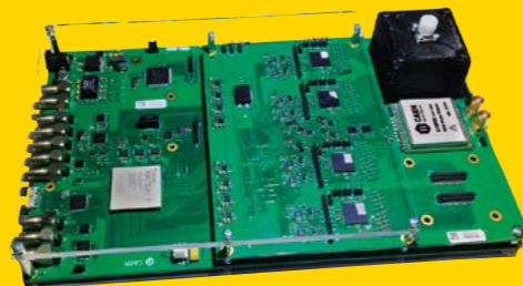
DT5550W 128 Channel SiPM Readout System
